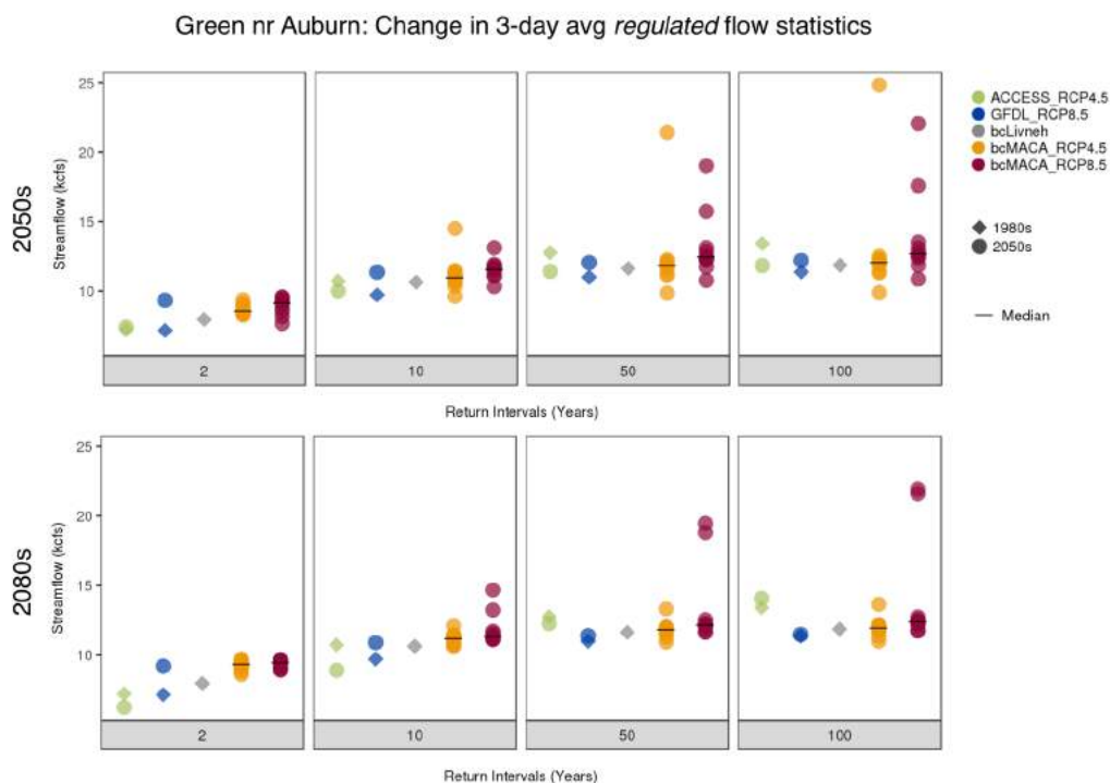
Figure 6.11 Future and historical flood statistics (2-, 10-, 50- and 100- year floods) using regulated flows for the Green River near Auburn. The plots include results for all DHSVM simulations for the 2050s (top) and 2080s (bottom). Historical flood statistics are based on water years 1971-1999
